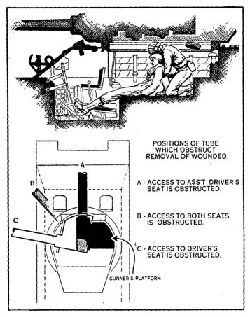
Figure 18. Removal of driver through the turret.
